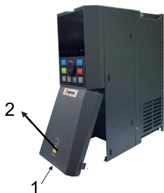
Figure3-6 Terminal cover's disassembly
